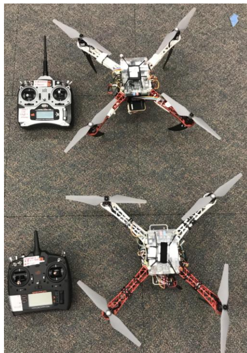
Figure A-4: Quads with controllers (new quad is bottom quad, it has thinner top plate and black ESCs)
